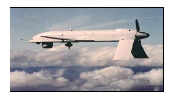
In our heightened military climate, long-range UAVs are in extremely high-demand for reconnaissance and surveillance because they can loiter for 24 hours or more at altitudes of over 65,000 feet and deliver high-quality synthetic-aperture-radar (SAR) images in real time to surface platforms.
