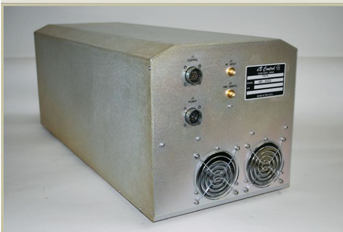
Figure 3: Designed for use in military manned and unmanned airborne applications, the dB-4522 TWT amplifier operates in the 11-18 GHz frequency range and provides 450W CW (at 11-17.5 GHz) and 400W CW (at 17.5-18 GHz) peak output power.
