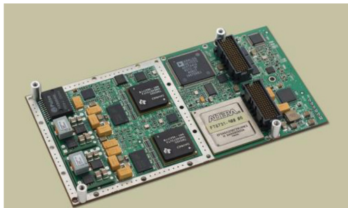
Figure 2: The ICS-8580 Rugged Video Streaming XMC supports numerous video formats with either two channels of high definition video or four channels of standard definition video. It provides an industry standard H.264 video compression codec, but is software-reconfigurable to enable it to support alternatives such as JPEG2000.
