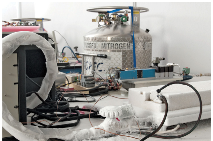
Figure 5: Liquid nitrogen is used to simulate extreme cold temperatures
