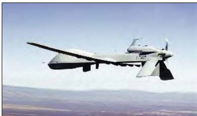
The MQ-9 Reaper can remain in the air for 35 hours at altitudes of more than 65,000 feet.
