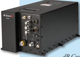
transmitters and EW threat simulators for manned and unmanned platforms. The dB-4410 weighs 70lb and measures 10.71 x 8.89 x 19.33 inches, including liquid cooling in the standard model, with alternative cooling methods available as customizable options.
