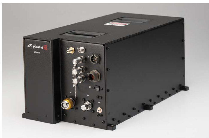
2. Model dB-4410 is a liquid-cooled amplifier module capable of 300 W CW output power from 7.5 to 18.0 GHz with 57-dB minimum gain.
