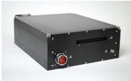
*The dB-9001 is a custom-mounted Instantaneous Frequency Measurement (IFM) unit operating in the C, X and Ku-band frequency range providing highly accurate measurements at 100 nanoseconds (ns) to CW pulse width measurements. The IFM units measure frequency, as well as power level and pulse duration. The IFM units are packaged in a custom configuration with integral forced-air and conduction cooling.*
